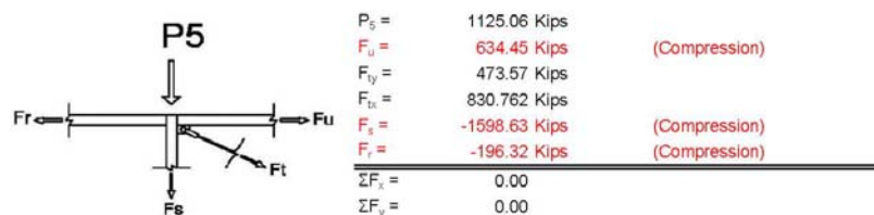
Calculations 5 through 9: Forces in Truss 2 Members
