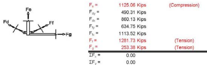
Calculations 1 through 4: Forces in Truss 2 Members
